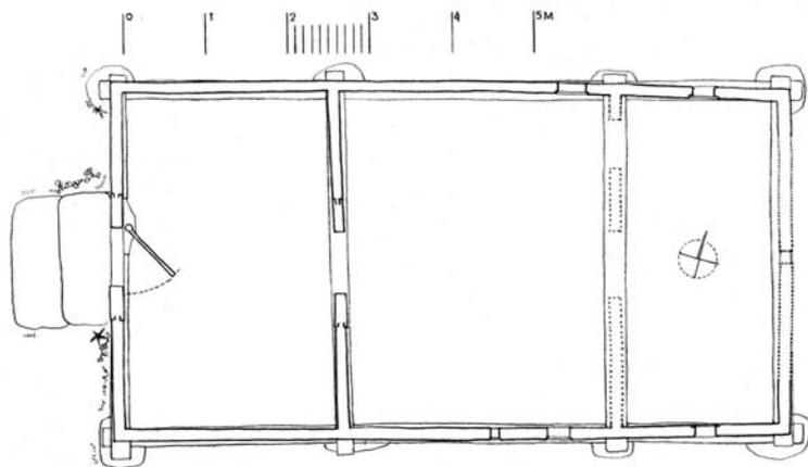
**115** *Valea Stejarului*. This is the single very small wooden church that survived, being only limitedly affected by extensions from the beginning of the 19th century. The church had a very simple oblong plan, just like in a common house, though the passages are oriented eastwards, as required by the ritual. Section through the former sanctuary, reconstruction of the southern façade and plan. Scale drawings: May 1996.
