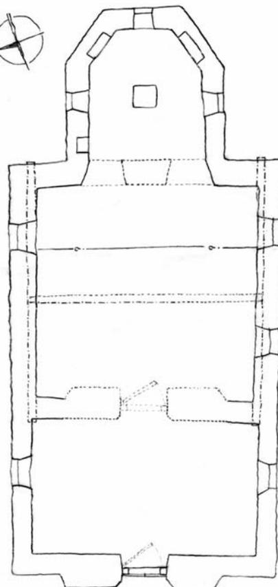
**235** *Sarasău*. The interior was also affected by the renovations from 1937, especially due to the demolition of the inner walls and the enlargement of the windows. Scale drawings of the section through the nave and the plan: October 2001.
