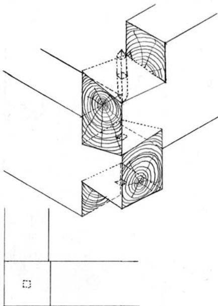
**56** *Poenile de sub Munte*. A particular type of dovetail joint with a recess inside. Scale drawing: June 1998.
