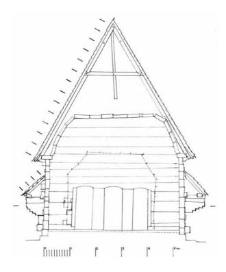
**92** *Corneşti.* The raftering and the vault share the same massive lateral purlins. Scale drawing of the section through the nave facing east: August 1997.
