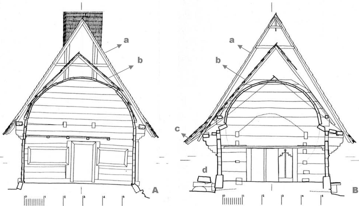
**88** *Breb* (A) and *Sârbi Susani* (B). Sections through the naves. In both churches the new roofs (a) took over the function of the earlier roofs (b). In *Sârbi Susani*, the short lower rafters (c) extended long outside to protect the ancestors' tables (d). Scale drawings from April-May 1995.
