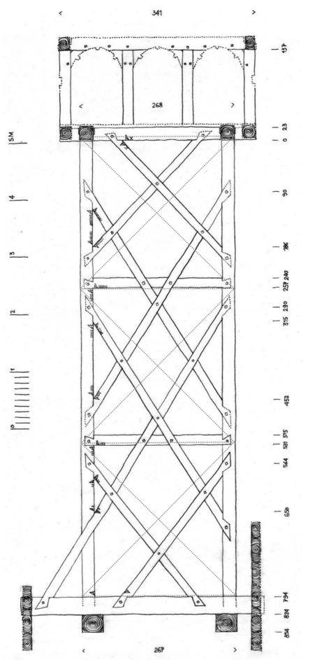
Sat Şugătag. The height of this tower was dimensioned 3 times its width which in its turn was established after the length of the narthex. Scale drawing of the southern side: October 2001.
