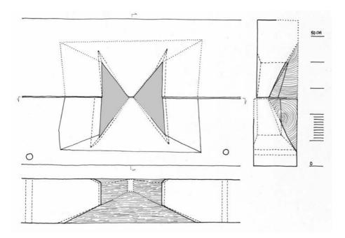
73 Cornești. Two logs from the northern wall of the church retain the halves of one or possibly two separate open windows. The samples taken from the logs gave firm dendrochronological no dating, but the windows seem to come from a previous construction, maybe from the 16th century. Scale drawings with а possible reconstruction, front side and sections: August 1997.
