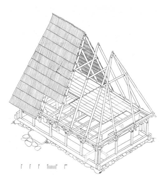
84 Călinești. The large house of the noble Tivadar family, probably dating from the turn of the 18th century, is an excellent example of а log construction built with double-slot joints. The steep roof is partly unloading through the log structure partly through the posts on two sides of the narrow Scale porch. drawing: October 2000.
