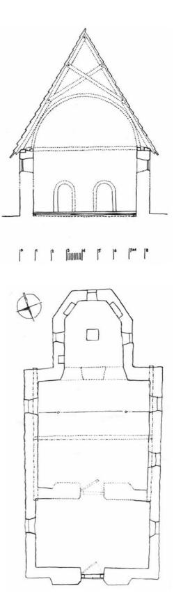
**235** *Sarasău*. The interior was also affected by the renovations from 1937, especially due to the demolition of the inner walls and the enlargement of the windows. Scale drawings of the section through the nave and the plan: October 2001.
