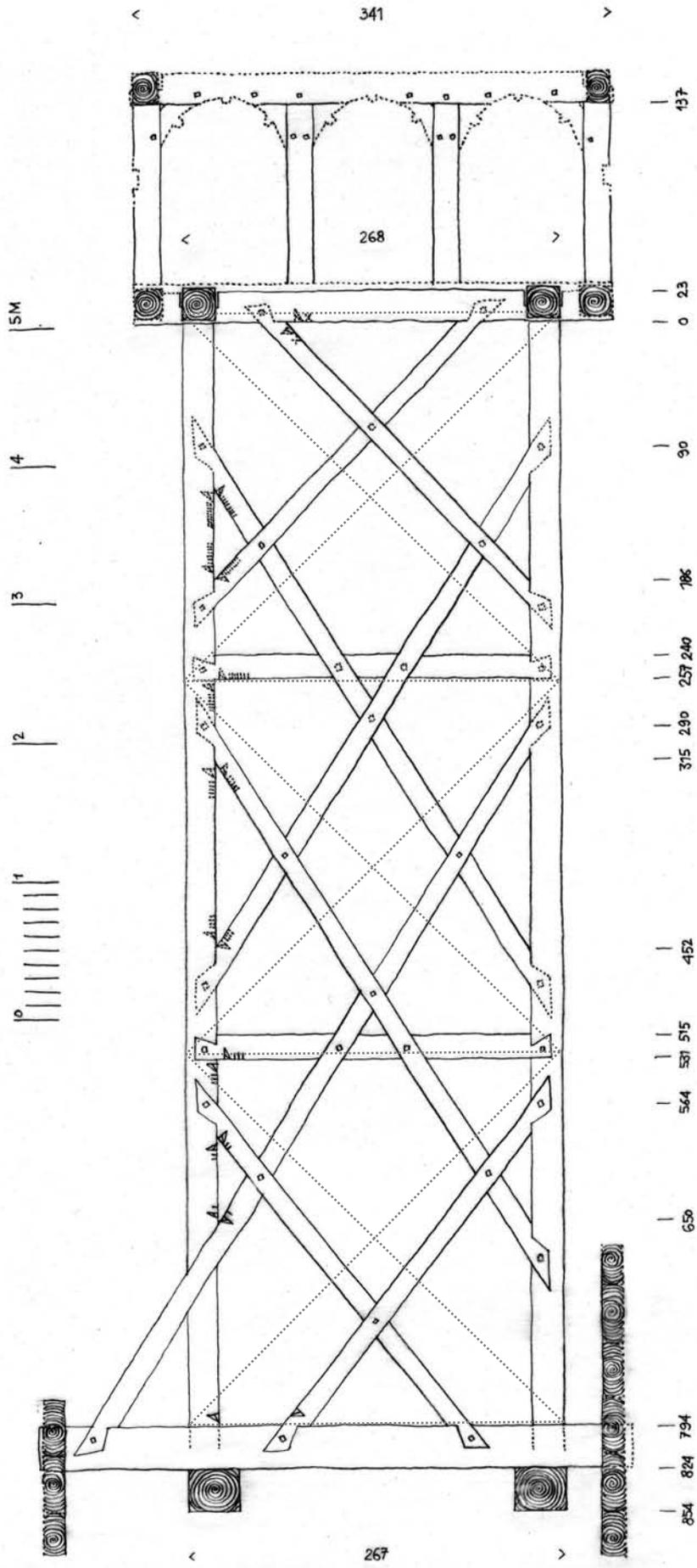
**113** *Sat Şugātag*. The height of this tower was dimensioned 3 times its width which in its turn was established after the length of the narthex. Scale drawing of the southern side: October 2001.
