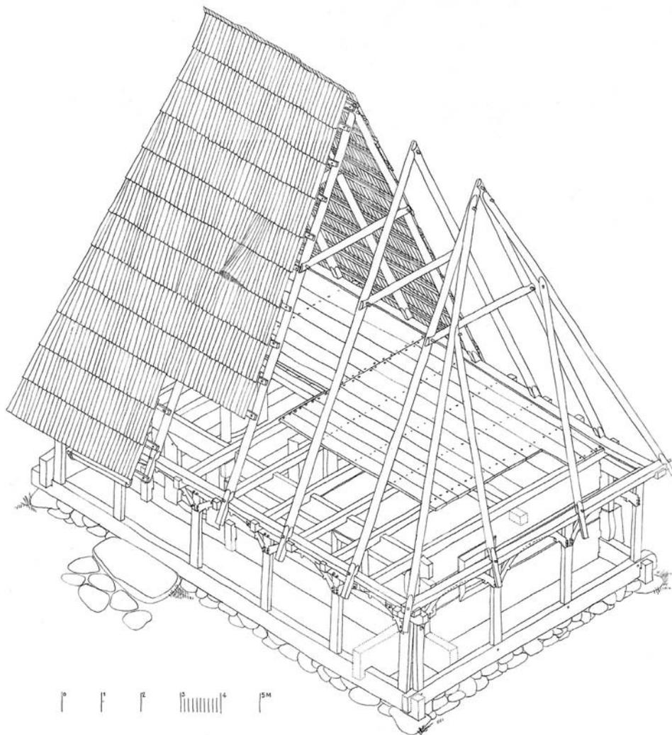
**84 Călinești.** The large house of the noble Tivadar family, probably dating from the turn of the 18th century, is an excellent example of a log construction built with double-slot joints. The steep roof is partly unloading through the log structure partly through the posts on two sides of the narrow porch. Scale drawing: October 2000.
