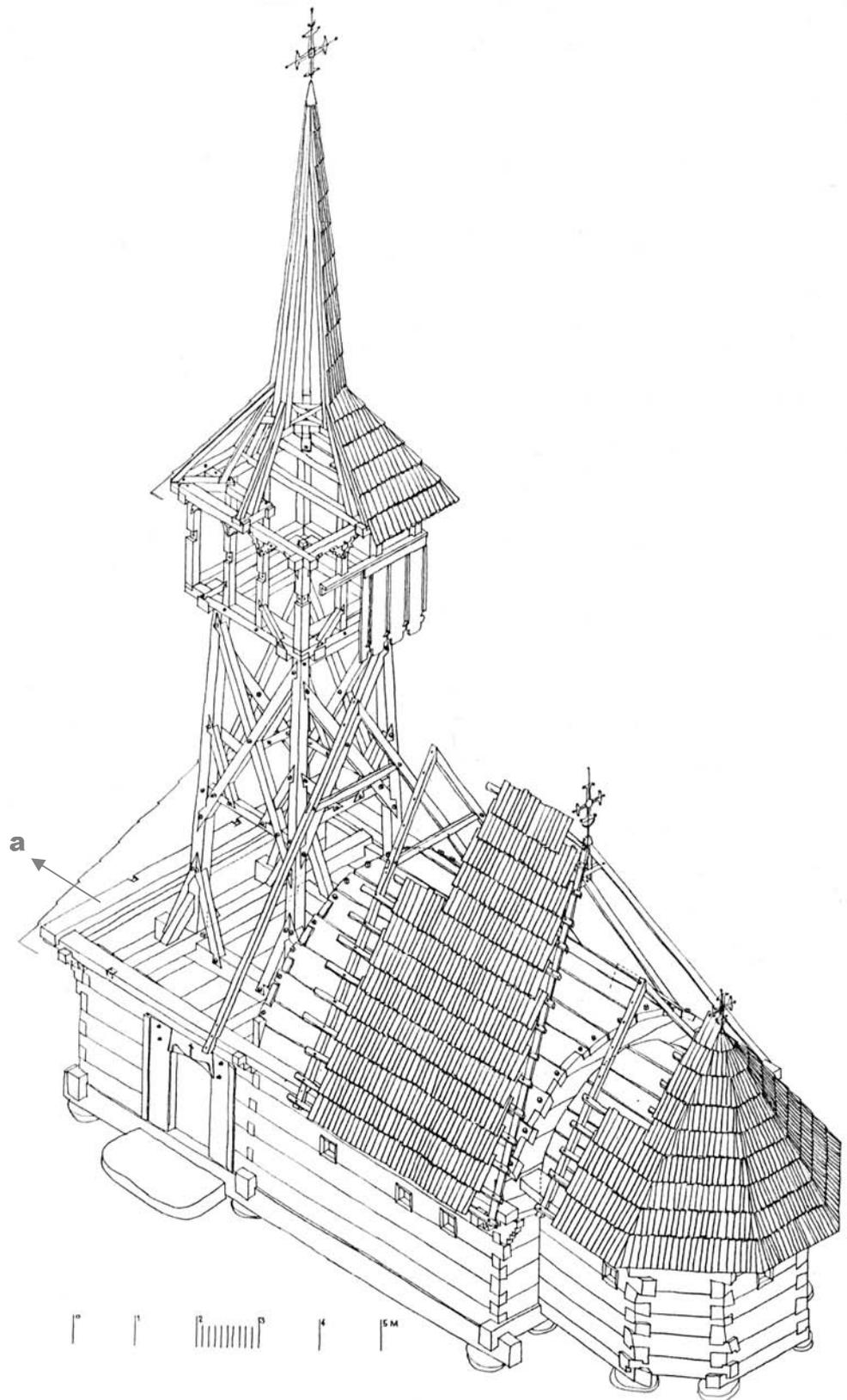
**86** *Călinești Căeni*. Axonometric reconstruction of the initial church and its simple roof. The eaves purlins jettied on consoles (a) goes all around the log fabric to support both the large roof above the church and the smaller one protecting the sanctuary. Scale drawing: August 1994.
