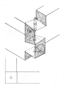
**56** *Poienile de sub Munte*. A particular type of dovetail joint with a recess inside. Scale drawing: June 1998.
