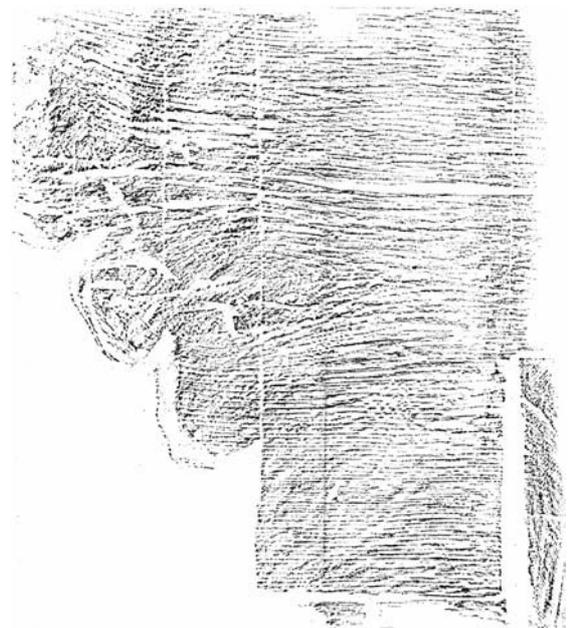
**159** *Sokyrnytsia*. The church carpenter liked to round off the serrated profile of the consoles. The working lines are still traceable on one of them. Tracing at the scale 1:4, July 1998.
