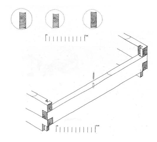
49 Botiza. The squared wall beams of the vanished church from Botiza (1594), exposed after the demolition of a former confessional school in Hoteni, were all cut lower than the round log would have allowed and decentred. seemingly with the intention to place the heart of the tree inside the hook Reconstructions of a squared log in the eastern wall of the sanctuary and of 3 sections through logs. Scale drawings August 1997 from and October 2000.
