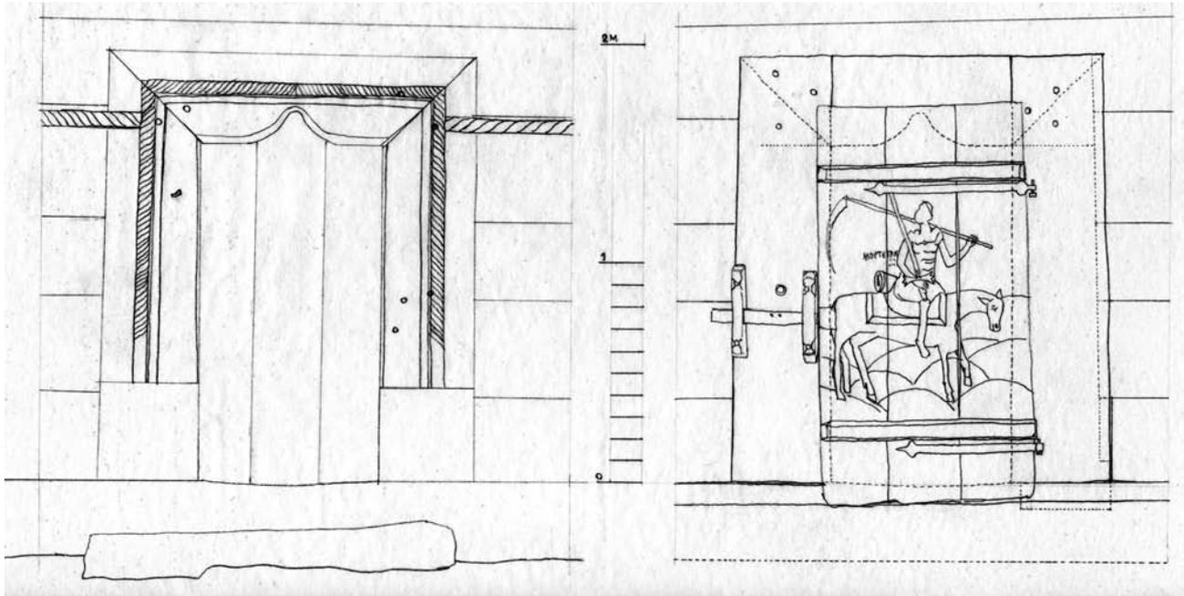
**65 Cuhea.** The front and the back of the entrance door survived in good condition. While the front is dominated by decorative carvings the back retains the functional parts: the wooden door bolt, iron hinges and fillets. The joining of the lintel with the lateral jambs shifts from flaring upwards at the front to straight at the back. Also remarkable is the painting of the riding Death on the backside of the door's leaf. Scale drawing: June 1998.
