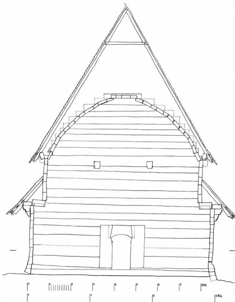
**91 Budești Josani.** A section through the largest known church room of wood from Maramureș in the past (above) uncover the problem at the upper eaves purlins, as they appeared twisted out of their position by the heavy roof. The solution was to build a gallery under the eaves purlins to unload them to the lower joints (below). If the galleries were built from the beginning the upper eaves purlins would have more effectively worked laid horizontally. Scale drawing and picture from August 1997.
