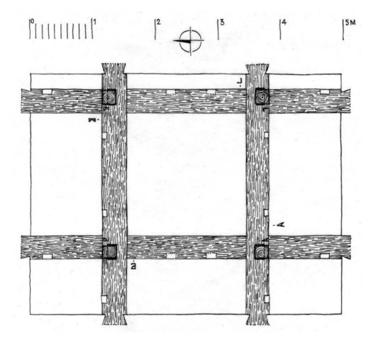
**141** Sat Şugătag. The base of the tower and the assembly marks used to distinguish the pieces from each side. Scale drawing: October 2001. **142** Darva (Kolodne). Although we lack a firm dating this seem to be, however, one of the oldest portals preserved in Maramureş. Scale drawing: October 2000.
