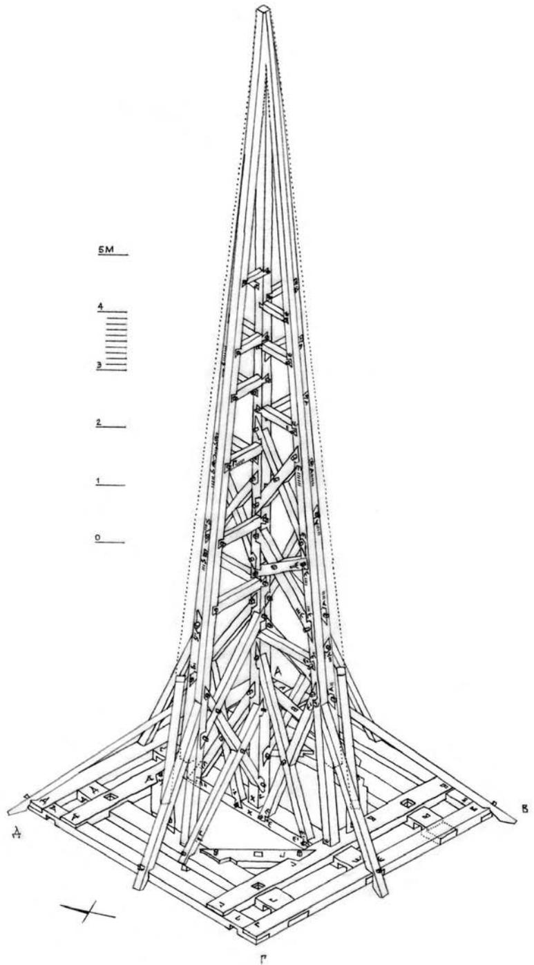
131 *Cuhea*. Commonly, a spire was very simply built of rafters and some rare cross braces and struts, but the slender spire from *Cuhea* displays one of the most complex structures, where the carpenter had to make use of assembly marks to differentiate the numerous parts. Scale drawings: June 1998.
