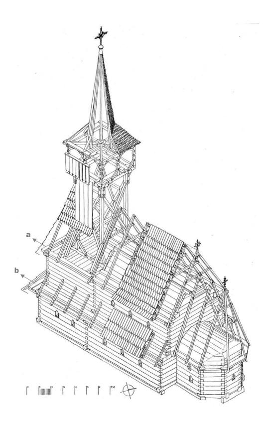
**90** *Ieud Deal*. Axonometric view with a reconstruction of the old lathing and shingling. Both the upper eaves (a) and the lower eaves (b) surround the log fabric on three sides and ends levelled with the eastern gable. The rafters over the small sanctuary were mainly sized in relation to the larger roof and secondarily with the width of the sanctuary. Scale drawing: July 1997.
