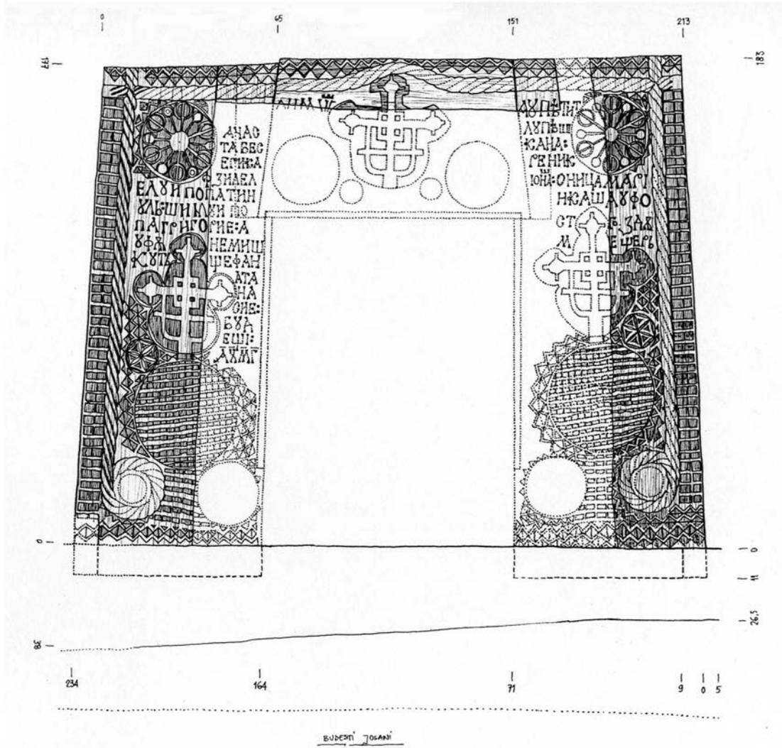
178 *Budești Josani*. Reconstruction of the portal of the entrance (above) and the signature of the master Gozdă (below). The inscription was partially composed after Bârlea 1909, 60/206, partly completed with the visible words on the right jamb. Remarkably, the close relation between lower crosses and sun-rosettes representing the two solstices was accentuated. Scale drawing and tracing 1:20, 1999.
