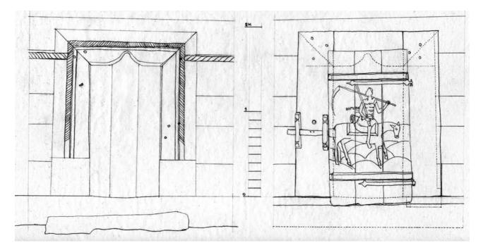
**65** *Cuhea.* The front and the back of the entrance door survived in good condition. While the front is dominated by decorative carvings the back retains the functional parts: the wooden door bolt, iron hinges and fillets. The joining of the lintel with the lateral jambs shifts from flaring upwards at the front to straight at the back. Also remarkable is the painting of the riding Death on the backside of the door's leaf. Scale drawing: June 1998.
