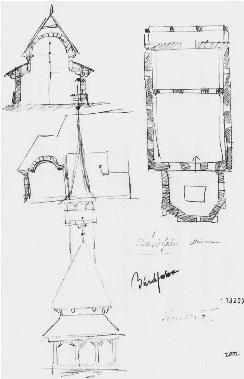
3 *Berbești*. Sketches signed by Ferencz Schulcz in 1862 representing a cross section through the nave, a partial longitudinal section through the sanctuary and nave, the plan and the western front. The value of these sketches increased after the demolition of the church in the summer of 1932. KÖH, Tervtár, K 2001.
