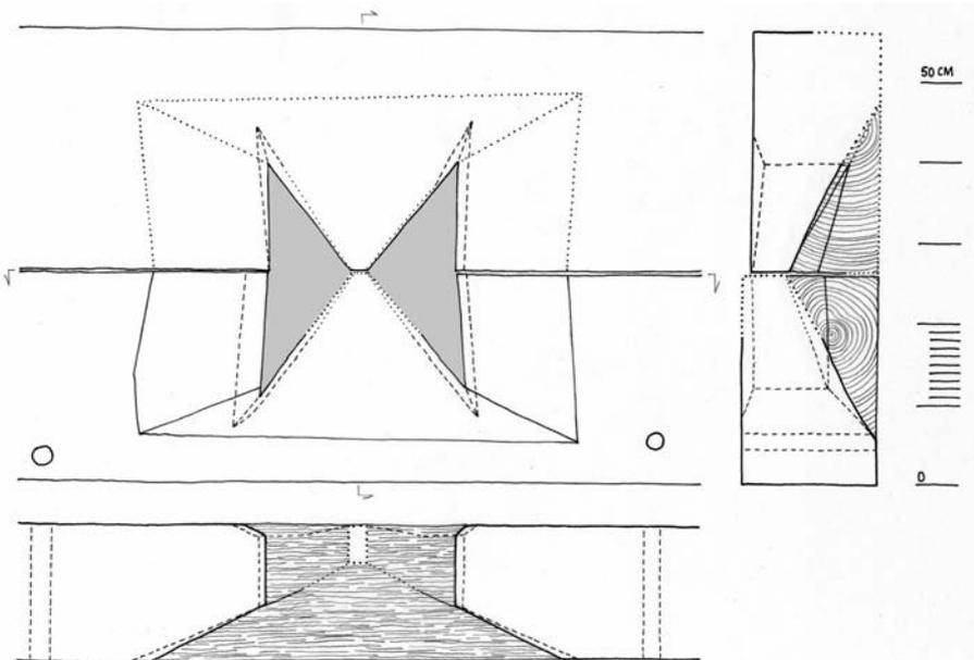
**73** *Cornești*. Two logs from the northern wall of the church retain the halves of one or possibly two separate open windows. The samples taken from the logs gave no firm dendrochronological dating, but the windows seem to come from a previous construction, maybe from the 16th century. Scale drawings with a possible reconstruction, front side and sections: August 1997.
