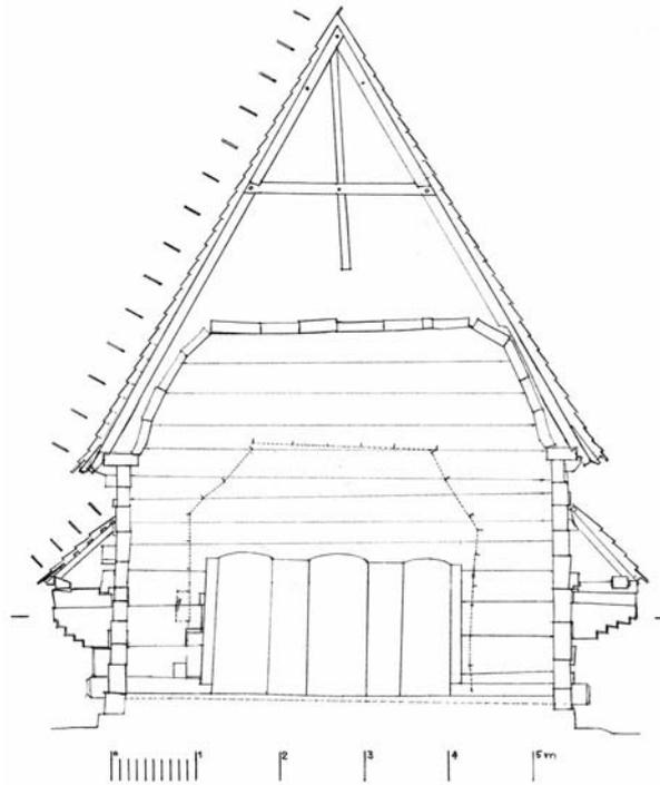
**92** *Cornești*. The raftering and the vault share the same massive lateral purlins. Scale drawing of the section through the nave facing east: August 1997.
