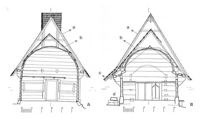
**88** *Breb* (A) and *Sârbi Susani* (B). Sections through the naves. In both churches the new roofs (a) took over the function of the earlier roofs (b). In Sârbi Susani, the short lower rafters (c) extended long outside to protect the ancestors' tables (d). Scale drawings from April-May 1995.
