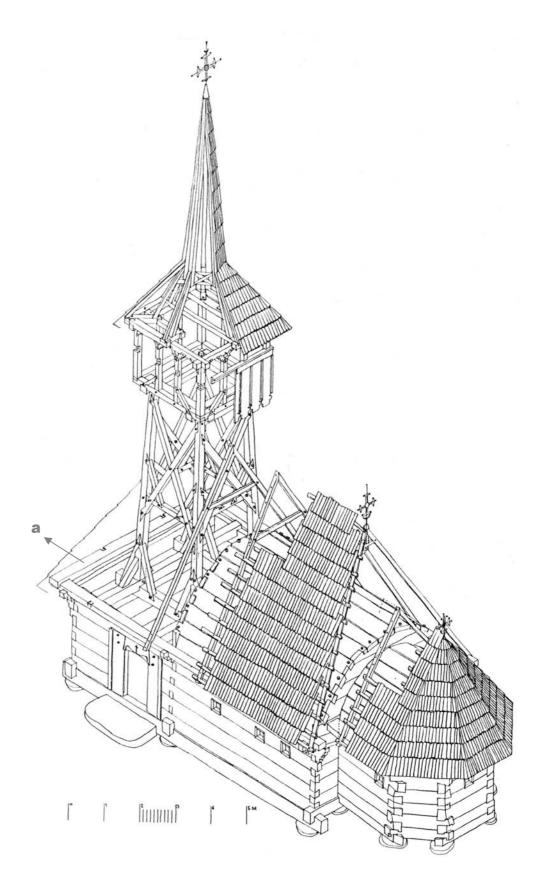
*Călineşti Căeni*. Axonometric reconstruction of the initial church and its simple roof. The eaves purlins jetted on consoles (a) goes all around the log fabric to support both the large roof above the church and the smaller one protecting the sanctuary. Scale drawing: August 1994.
