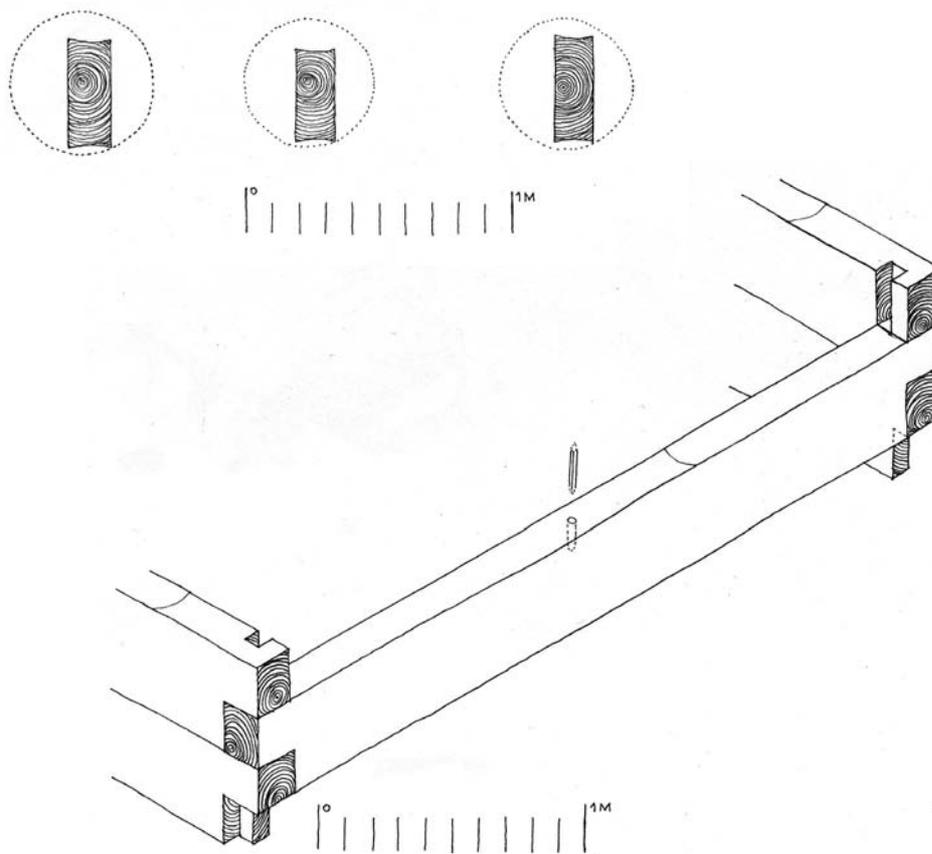
49 *Botiza*. The squared wall beams of the vanished church from Botiza (1594), exposed after the demolition of a former confessional school in Hoteni, were all cut lower than the round log would have allowed and decentred, seemingly with the intention to place the heart of the tree inside the hook. Reconstructions of a squared log in the eastern wall of the sanctuary and of 3 sections through logs. Scale drawings from August 1997 and October 2000.
