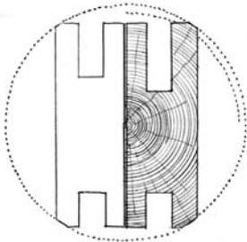
**69 Budeşti Josani.** The pair of jambs from the inner portal was cut from a single log, about 65 cm in diameter, split into two halves. Scale drawing: August 1997.
