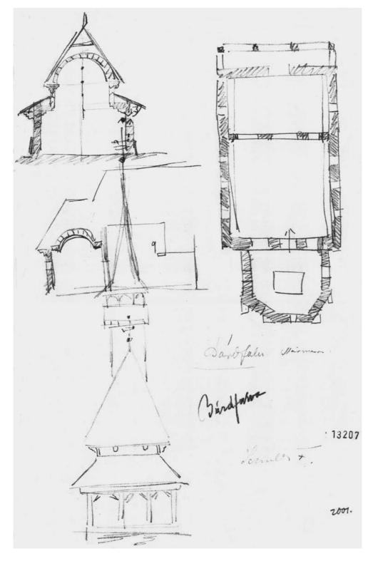
**3** *Berbeşti*. Sketches signed by Ferencz Schulcz in 1862 representing a cross section through the nave, a partial longitudinal section through the sanctuary and nave, the plan and the western front. The value of these sketches increased after the demolition of the church in the summer of 1932. KÖH, Tervtár, K 2001.
